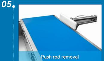
Eliminate non-conforming products through push rod method, suitable for most small or large packaging
