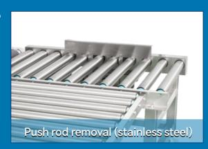
Using metal push rods to remove non-conforming products, suitable for hard packaging and box packaging 04.
