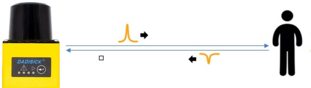
Figure 3-1 schematic diagram of lidar ranging principle
