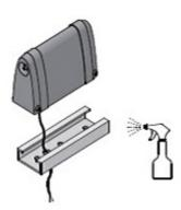
7. For safety edges with C-shaped bases, one side must be snapped into the mounting base and then pressed into the entire C-shaped base. Pushing and pulling the safety edge in the mounting base will cause damage to the safety edge and should be avoided at all costs.
