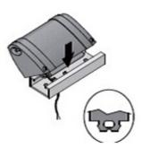
8. For safety edges with T-shaped bases, insert them from the side along the groove of the mounting base.
