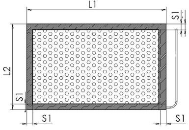
Effective area of standard safety mat:  $L1 \times L2 \leq 1.5 \text{ m}^2$ . For the protection area more than 1.5 m2, it is recommended to adopt the assembly method of multiple safety mats.
