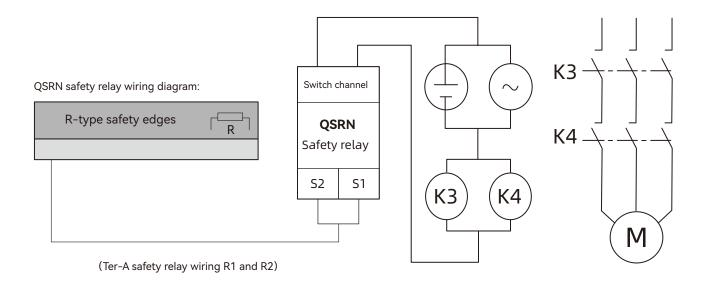
2) Sensing output - a combination of multiple safety edges connected in series R/K series combination of safety edges
