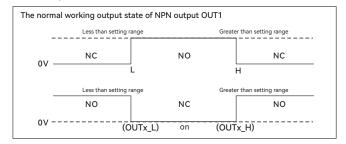
Note \* When working normally, OUT1 or OUT2 is set to NC, The L-H interval maintains NPN output continuously, while other areas are disconnectedState; When OUT1 or OUT2 is set to normally open, The L-H interval remains disconnected, while other areas maintain NPN output.
