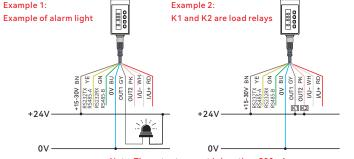
Note: The output current is less than 500mA
