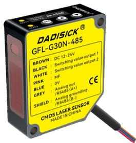
The detection angle needs to be perpendicular to the measured object within  $90^\circ \pm 15^\circ$ . Transparent objects cannot be detected, liquids cannot be detected, and the range cannot be calculated from 0.
