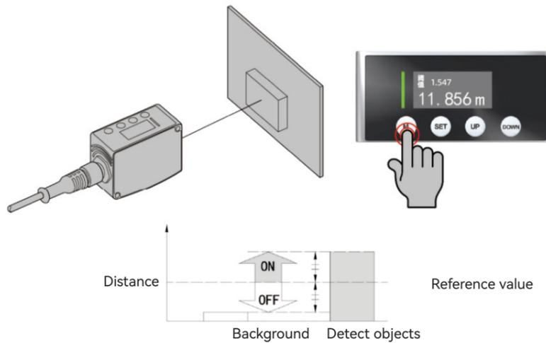
③ Calibration completed. (When the difference between the two teachings is small, the display return difference is too small, and you need to increase the difference and teach again)
