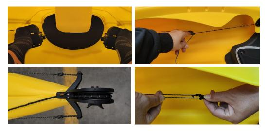
6. When the rudder foil is down vertically, it's ready to use
