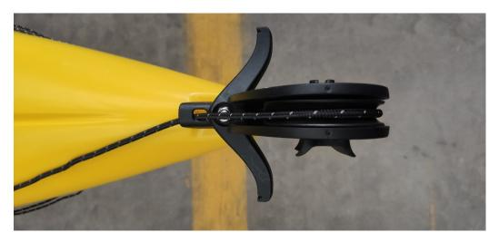
4. Insert the rudder steering rope through the rudder house hole, hook back and tighten it, do same on the other side of the rudder
