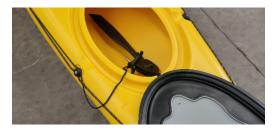
3. Check the rudder pin lock direction, slide in the rudder pin correctly till the bottom, and spin the rudder in position
