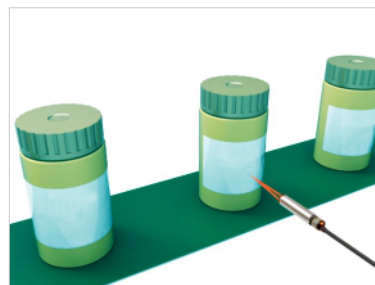
Detecting the presence of packaging bottles
