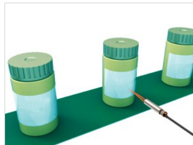
Detecting the presence of packaging bottles
