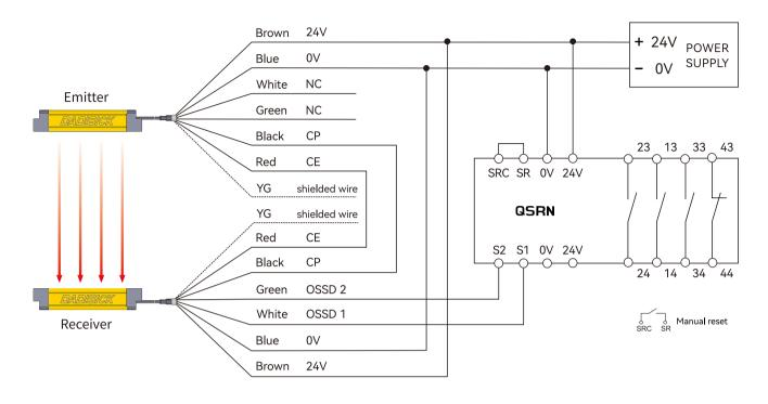
2. Optical synchronous safety light curtain connection QSRN safety relay wiring diagram
