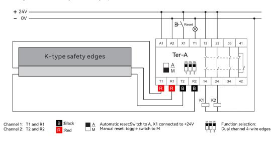
2) Sensing output - a combination of multiple safety edges connected in series R/K series combination of safety edges
