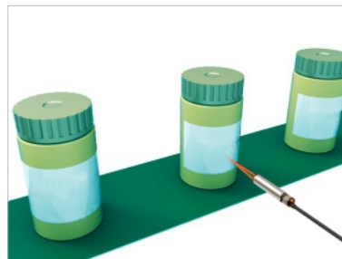
Detecting the presence of packaging bottles
