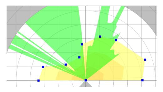
There are 64 channels in the sensor, and up to 64 different sensing ranges can be set. Meet the detection needs in different occasions. The following figure shows the AGV application process.
