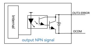
The output ports are all NPN outputs. Please refer to the following figure for the output schematic:
