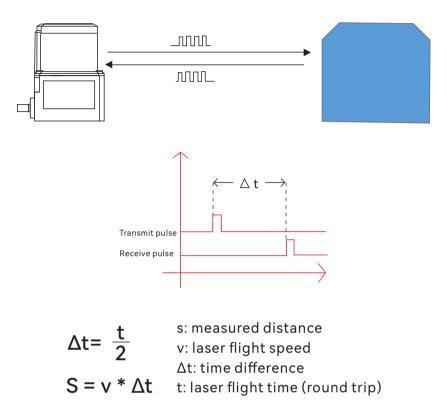
The laser beam is used to perform a two-dimensional scan of the surroundings to obtain an environmental contour graphic. The protection area range is established through software configuration. Once an object is in the set area, the sensor will have a corresponding output port signal output. After the upper computer obtains the signal, it will make further judgments and processing.
