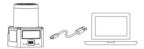
Notice Connecting the data cable to the sensor end in the wrong direction will damage the sensor port. You must use a cable that can transmit data. The charging cable cannot be connected successfully.
