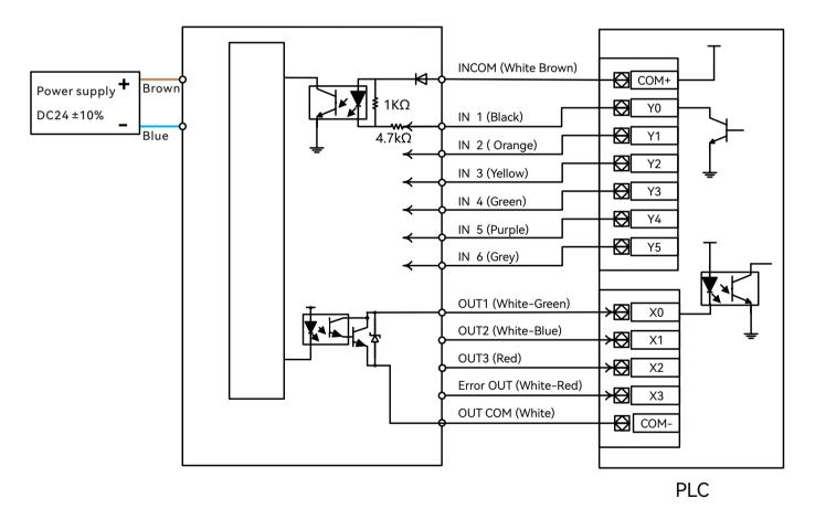
X0-3 is the signal input port of PLC; Y0-Y5 are the signal output ports of PLC; IN1-IN6 input current is greater than 10mA; Out1-Out4 output current is less than 100mA;
