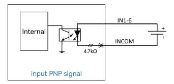
The sensor has 64 channels, and the input signal combination is switched to the specified channel number through 6 IO ports. The detection range of the channel needs to be set in advance through the configuration software. The external device selects and switches the area through the input signal.
