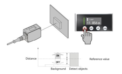
③ Calibration completed. (When the difference between the two teachings is small, the display return difference is too small, and you need to increase the difference and teach again)
