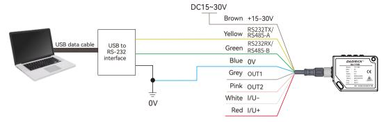
Note: RXD and TXD on the computer side and instrument side need to be cross-connected. RS232 has three connections: RX (green) TX (yellow) GND (blue).
