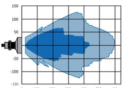
Figure 11 - CSB30-6000 Ultrasonic Propagation area
