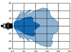
Figure 9 - CSB30-2000 ultrasonic wave propagation area
