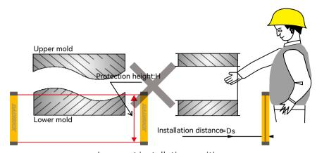
Incorrect installation position (light curtain is low, human hand can reach out from the top of the light curtain)
