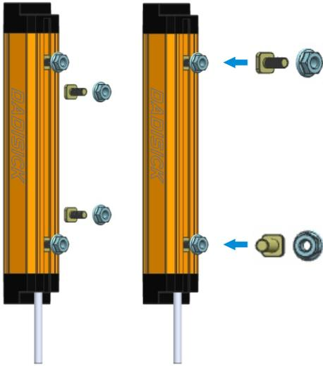
1. Installation method of T-shaped screws on the back
