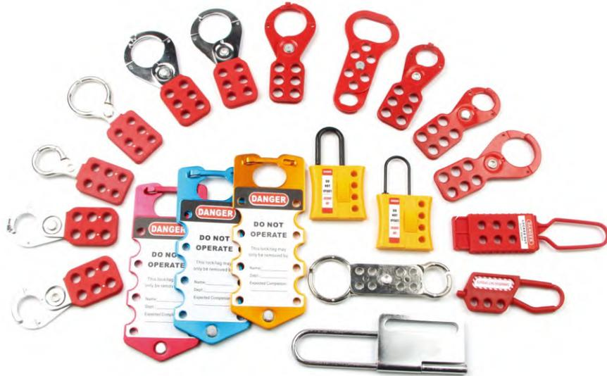
Lockout Hasps are a neat and convenient way to lockout an energy source ensuring that your worker's safety is never compromised. The hasp is fitted to the isolation point. The multiple workers can apply their lockout padlock.
