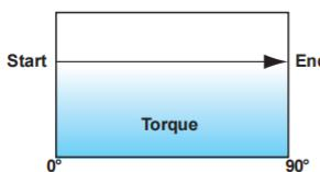
Spring Return Torque Output Diagram
