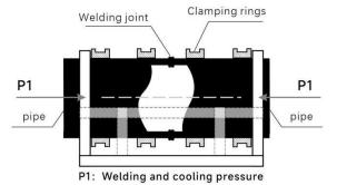
Allow joint to cool under pressure according
