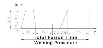
**t1 Phase:** Pressure P2 works on the fusion interface, the purpose is to erase the distance between the pipe ends and heater so that the whole pipe ends can be heated in balance. That' why in this phase, there is no precise time for evaluation, it is checked according to the fusion loop height.
