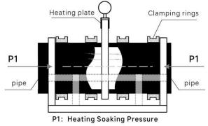
Ensure the heater stays perpendicular to the pipe by supporting the heater during the heating process.
