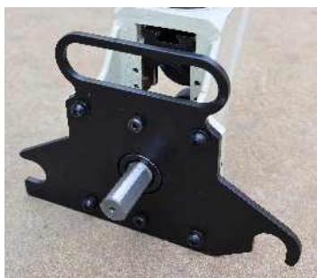
*Adapter plate to fit on threading machine
