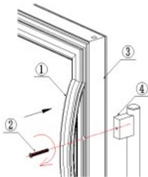
① First remove the gasket from the groove of the door ②
