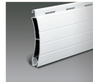
Name: 55mm double layer slat Thickness: 11.3mm Weight: 5.9Kg/m 2 Maximum width: 4.0m Maximum height: 3.5m Maximum area: 12m 2 Quantity of per meter height: 18 pcs Surface treating: powder coating Color: Yellow wood, dark wood (Other color can be made upon customer's request.) Pattern: unperforated, perforated (2%)
