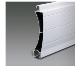
Name: 77 double layer slat Thickness: 18.4mm Weight: 6.9Kg/m 2 Maximum width: 6.5m Maximum height: 6.5m Maximum area: 35m 2 Quantity of per meter height: 13pcs Material: 0.3mm Aluminum plate Surface treating: Baking finish Color: White, Beige, Grey (Other color can be made upon customer's request.) Pattern: unperforated
