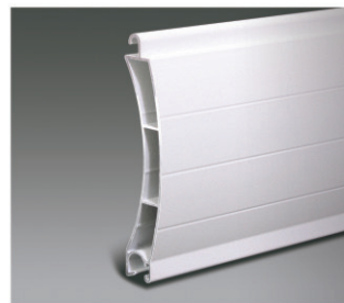
Name: 68mm double layer slat Thickness: 14.5mm Weight: 7.2Kg/m 2 Maximum width: 4.0m Maximum height: 5.8m Maximum area: 8m 2 Quantity of per meter height: 15 pcs Surface treating: powder coating Color: Yellow wood, dark wood (Other color can be made upon customer's request.) Pattern: unperforated
