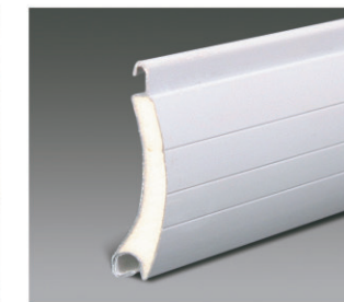
Name: 55 mm foam slat Thickness: 12.5mm Weight: 4.6Kg/m 2 Maximum width: 3.5m Maximum height: 4.2m Maximum area: 11m 2 Quantity of per meter height: 18pcs Material: 0.3mm Aluminum plate Surface treating: Baking finish Color: White, Beige, Grey (Other color can be made upon customer's request.) Pattern: unperforated, perforated (2%)
