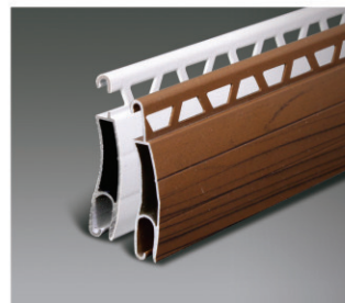
Name: 32mm double layer slat Thickness: 8.3mm Weight: 5.1Kg/m 2 Maximum width: 2.5m Maximum height: 3.0m Maximum area: 7m 2 Quantity of per meter height: 31 pcs Surface treating: powder coating Color: Yellow wood, dark wood (Other color can be made upon customer's request.) Pattern: unperforated, perforated (2%,12%)
