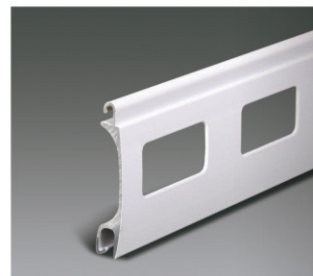
37mm single layer slat Thickness: 8.3mm Weight: 6.2Kg/m 2 Maximum width: 3.0m Maximum height: 3.0m Maximum area: 8m 2 Quantity of per meter height: 27 pcs Surface treating: powder coating Color: Yellow wood, dark wood (Other color can be made upon customer's request.) Pattern: unperforated, perforated (20%)
