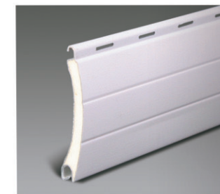
Name: 39 mm foam slat Thickness: 10mm Weight: 3.5Kg/m 2 Maximum width: 2.5m Maximum height: 3.0m Maximum area: 7m 2 Quantity of per meter height: 27 pcs Material: 0.3mm Aluminum plate Surface treating: Baking finish Color: White, Beige, Grey (Other color can be made upon customer's request.) Pattern: unperforated, perforated (2%)
