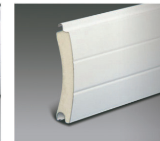
Name: 77 mm foam slat Thickness: 20.0mm Weight: 5.0Kg/m 2 Maximum width: 5.5m Maximum height: 4.2m Maximum area: 18m 2 Quantity of per meter height: 13pcs Material: 0.46mm Aluminum plate Surface treating: Baking finish Color: White, Beige, Grey (Other color can be made upon customer's request.) Pattern: unperforated
