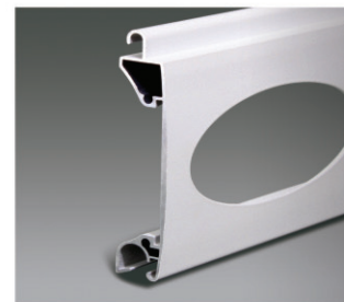
Name: 77 single layer slat Thickness: 17.5mm Weight: 8.0Kg/m 2 Maximum width: 5.5m Maximum height: 4.0m Maximum area: 20m 2 Quantity of per meter height: 13pcs Material: 0.3mm Aluminum plate Surface treating: Baking finish Color: White, Beige, Grey (Other color can be made upon customer's request.) Pattern: unperforated, perforated (20%)
