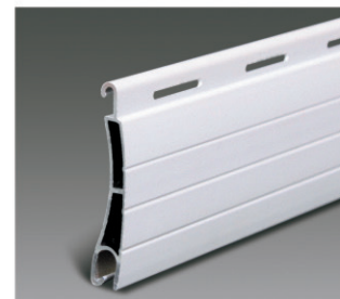
Name: 42mm double layer slat Thickness: 10mm Weight: 5.7Kg/m 2 Maximum width: 3.0m Maximum height: 3.0m Maximum area: 9m 2 Quantity of per meter height: 24 pcs Surface treating: powder coating Color: Yellow wood, dark wood (Other color can be made upon customer's request.) Pattern: unperforated, perforated (2%)
