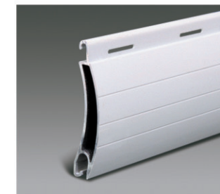
Name: 55mm double layer slat Thickness: 14mm Weight: 9.7Kg/m 2 Maximum width: 4.0m Maximum height: 3.5m Maximum area: 12m 2 Quantity of per meter height: 18 pcs Surface treating: powder coating Color: Yellow wood, dark wood (Other color can be made upon customer's request.) Pattern: unperforated, perforated (2%)
