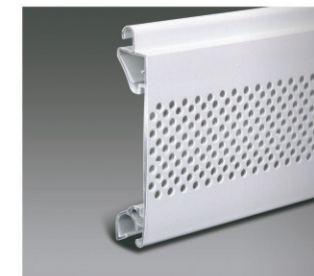
Name: 77 single layer slat Thickness: 17.5mm Weight: 8.0Kg/m 2 Maximum width: 5.5m Maximum height: 4.0m Maximum area: 20m 2 Quantity of per meter height: 13pcs Material: 0.3mm Aluminum plate Surface treating: Baking finish Color: White, Beige, Grey (Other color can be made upon customer's request.) Pattern: Micro-hole
