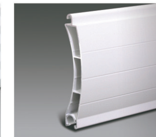
Name: 100 double layer slat Thickness: 22.4mm Weight: 6.3Kg/m 2 Maximum width: 7.0m Maximum height: 8.3m Maximum area: 40m 2 Quantity of per meter height: 10 pcs Surface treating: powder coating Color: Yellow wood, dark wood (Other color can be made upon customer's request.) Pattern: unperforated
