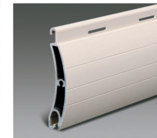
Name: 56mm double layer hurricane slat Thickness: 14mm Weight: 10.3Kg/m 2 Maximum width: 4.0m Maximum height: 3.5m Maximum area: 12m 2 Quantity of per meter height: 18 pcs Surface treating: powder coating Color: Yellow wood, dark wood (Other color can be made upon customer's request.) Pattern: unperforated, perforated (2%)
