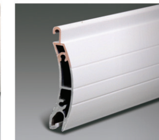
Name: 56mm double layer hurricane slat Thickness: 14.5mm Weight: 12.3Kg/m 2 Maximum width: 6.5m Maximum height: 4.0m Maximum area: 22m 2 Quantity of per meter height: 18 pcs Surface treating: powder coating Color: Yellow wood, dark wood (Other color can be made upon customer's request.) Pattern: unperforated
