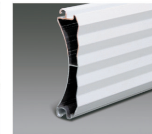
Name: 78 double layer slat Thickness: 18.6mm Weight: 6.6Kg/m 2 Maximum width: 6.0m Maximum height: 5.7m Maximum area: 30m 2 Quantity of per meter height: 13 pcs Surface treating: powder coating Color: Yellow wood, dark wood (Other color can be made upon customer's request.) Pattern: unperforated
