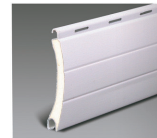
Name: 45 mm foam slat Thickness: 9mm Weight: 4.2Kg/m 2 Maximum width: 3.0m Maximum height: 4.0m Maximum area: 8m 2 Quantity of per meter height: 23 pcs Material: 0.3mm Aluminum plate Surface treating: Baking finish Color: White, Beige, Grey (Other color can be made upon customer's request.) Pattern: unperforated, perforated (2%)
