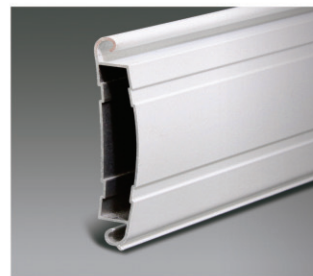
Name: 64mm double layer slat Thickness: 14mm Weight: 6.9Kg/m 2 Maximum width: 5.5m Maximum height: 4.0m Maximum area: 16m 2 Quantity of per meter height: 16 pcs Surface treating: powder coating Color: Yellow wood, dark wood (Other color can be made upon customer's request.) Pattern: unperforated
