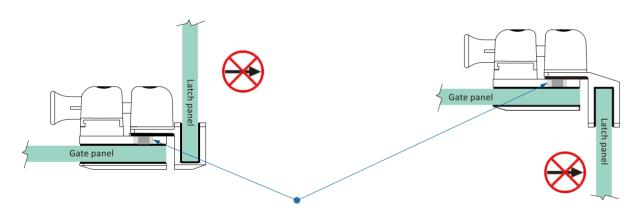
For Glass to Glass corner latch, we designed a safety hook which hooks into a slot in the backing plate for gate panel when the door is closed to prevent the latch from accidental un-latching when the latch panel is pulled outwards.
