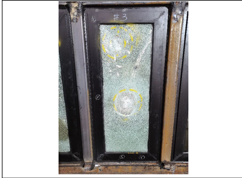
Photo No.5 Specimen #3 after cyclic test (Testing on December 21, 2021)
