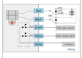
Set SW to [OPEN] - the red wire connect to the (+) pole of power supply, the black wire connect to the (-) pole of power supply, and connect the green wire with fully-open control terminal on the control device, the yellow wire with fully-closed control terminal, white wire is the common wire, when the electric valve fully opens, the green wire outputs valve-fully-open signal, with signal received, the SW is set to switch to STOP position, the valve stops action and keeps in fully open position.
