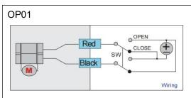
1. Set SW to [OPEN], the electric valve opens, and it stays in position after it is fully opened. The valve is de-energized (no power consumption).
