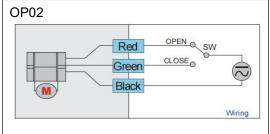
Both AC and DC power supply workable, while powered with DC power supply, connect the black wire to the (-) pole of power source.
