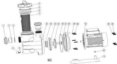
1. Joint nut 2. Joint 3.0 ring 4. Perspective cover spanner 5. Perspective cover 6.0 ring 7. Filter basket 8. Drainage plug 9.0 ring 10. Hexagonal bolt and flat washer 11. Base plate 12. Base plate rubber strip 13.0 ring 14. Diffuser 15. Impeller 16.0 ring 17. Mechanical seal 18. Cover plate 19. Bolt 20. Filta washer 21. Motor 22. Bolt 23. Flat washer
