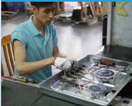
▼ 1st Flame test
