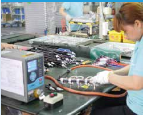
▼ 1st Gas leakage test
