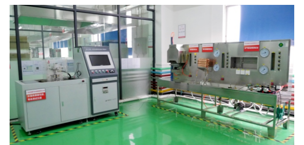
Burner, Heat Exchanger And Gas Valve Testing Equipment
