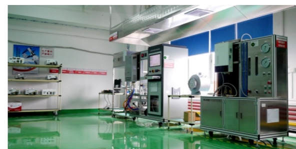
Water Heater Integrated Automatic Testing Equipment
