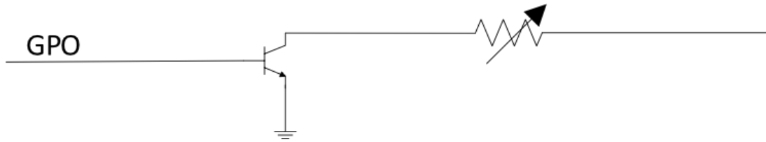
Figure 3-3 Internal Circuit of Output Signal
