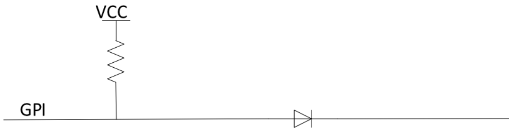
Figure 3-1 Internal Circuit of Input Signal
