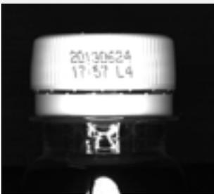
Imaging for characters printed on water bottle cap
