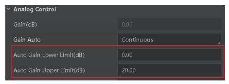
Figure 11-19 Set Gain under Once or Continuous Mode
