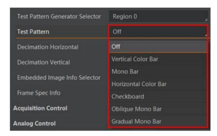
Figure 11-6 Set Test Pattern
