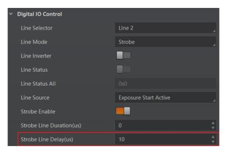
Figure 9-5 Set Strobe Line Delay
