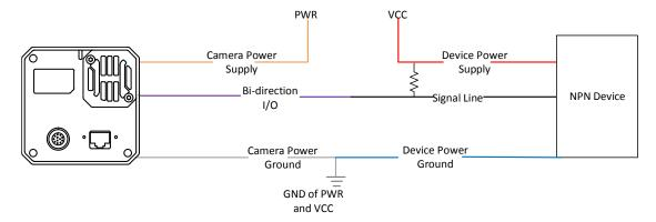
Figure 10-17 Line 2 Connecting to NPN Device as Output
