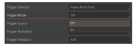
Figure 8-3 Set Trigger Mode
