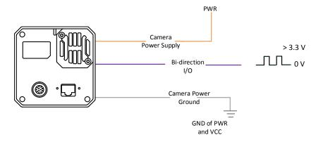
Figure 10-15 Line 2 Connecting to a Switch as Input
