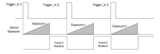
Figure 7-6 External Trigger Non-Overlap Exposure
