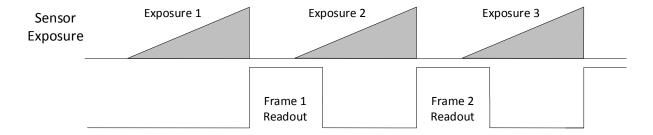
Figure 7-7 Internal Trigger Overlap Exposure
