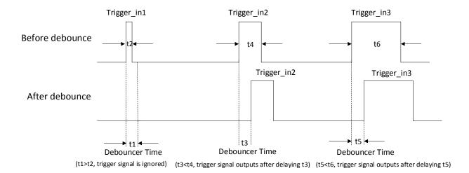
Figure 8-17 Trigger Debouncer Sequence Diagram
