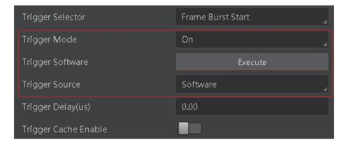
Figure 8-5 Set Software Trigger
