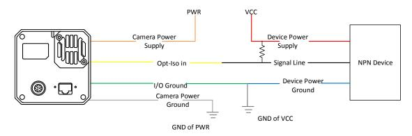
Figure 10-9 Line 0 Connecting to NPN Device
