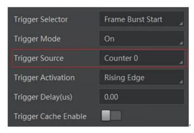
Figure 8-8 Set Counter Trigger
