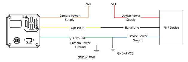
Figure 10-8 Line 0 Connecting to PNP Device
