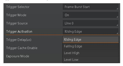
Figure 8-16 Set Trigger Activation
