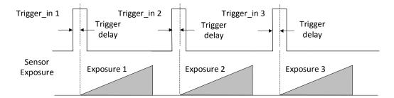
Figure 8-13 Signal Delay Sequence Diagram
