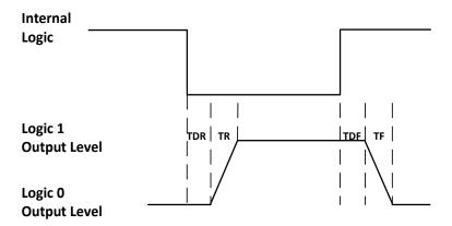
Figure 10-7 Output Logic Level
