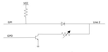
Figure 10-5 Line 2 Internal Circuit
