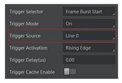
Figure 8-7 Set Hardware Trigger
