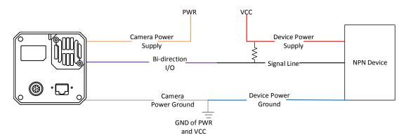
Figure 10-14 Line 2 Connecting to NPN Device as Input
