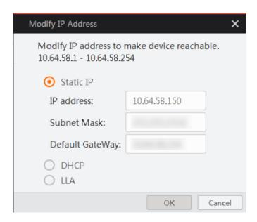
Figure 5-5 Modify Device IP Address
