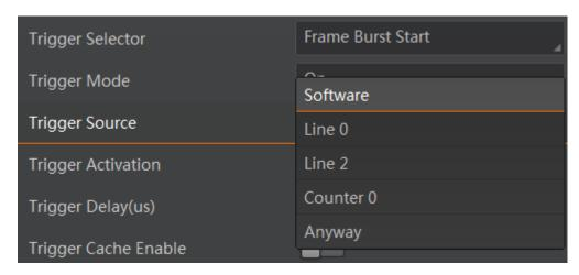
Figure 8-4 Set Trigger Source
