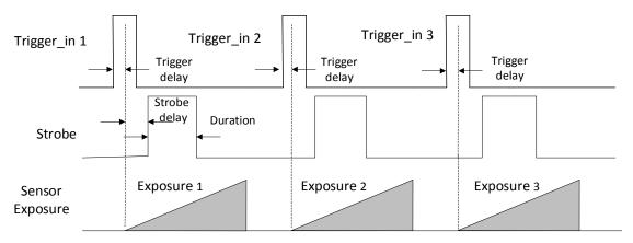
Figure 9-6 Sequence Diagram of Strobe Line Delay
