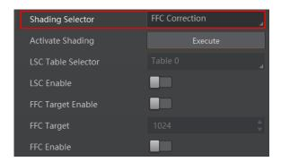
Figure 11-33 FFC Correction
