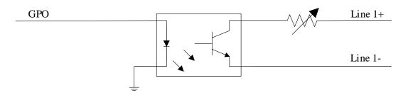
Figure 10-3 Line 1 Internal Circuit
