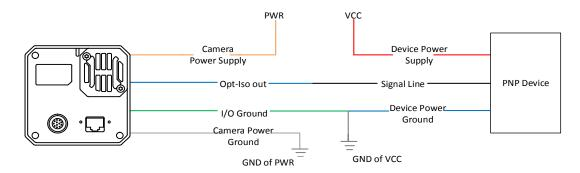
Figure 10-11 Line 1 Connecting to PNP Device
