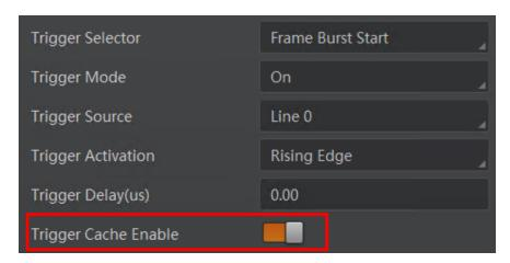
Figure 8-15 Enable Trigger Cache Enable
