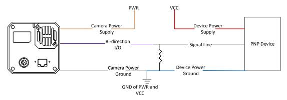
Figure 10-13 Line 2 Connecting to PNP Device as Input
