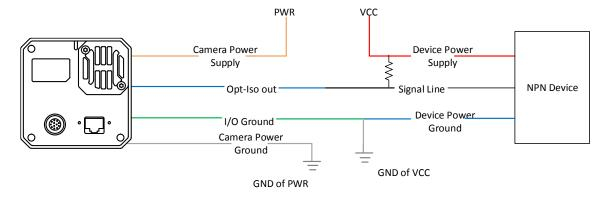
Figure 10-12 Line 1 Connecting to NPN Device
