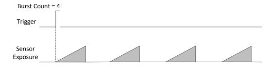
Figure 8-12 Sequence Diagram of Burst Frame Count
