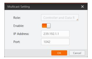
Figure 12-5 Set Multicast for Connected Camera
