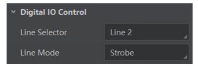
Figure 9-1 Set Line 2 as Output Signal
