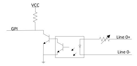
Figure 10-1 Line 0 Internal Circuit
