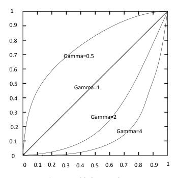
Figure 11-23 Gamma Curve
