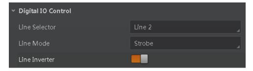
Figure 9-2 Enable Line Inverter
