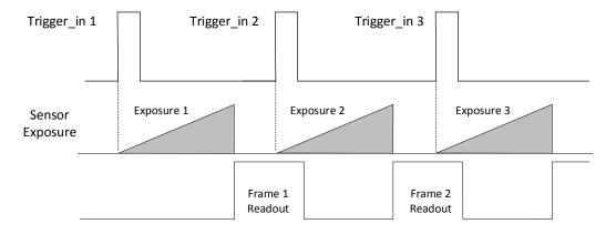
Figure 7-8 External Trigger Overlap Exposure
