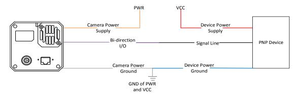
Figure 10-16 Line 2 Connecting to PNP Device as Output
