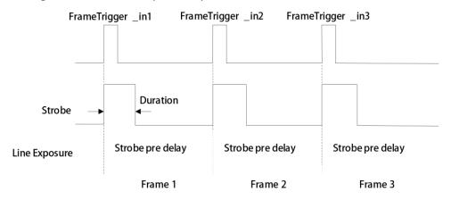
Figure 8-9 Sequence Diagram of Strobe Line Pre Delay
