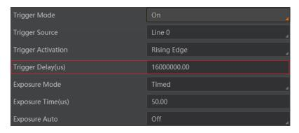
Figure 7-24 Set Trigger Delay
