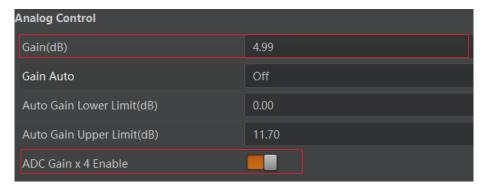
Figure 10-24 Set ADC Gain x 4 Enable
