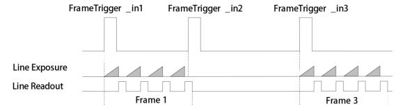
Figure 7-26 Second Frame Filtered
