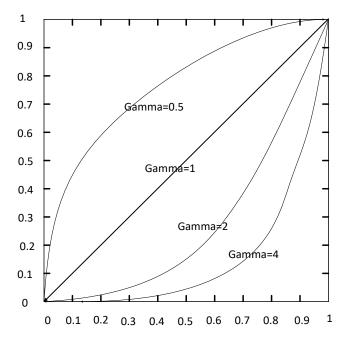
Figure 10-30 Gamma Curve
