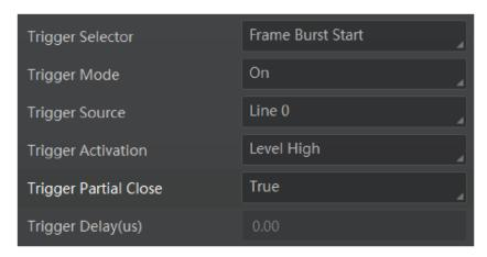
Figure 7-21 Level Trigger in Frame Trigger
