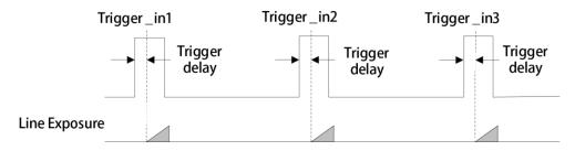
Figure 7-23 Signal Delay Sequence Diagram
