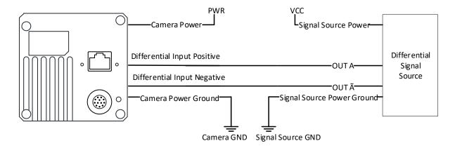
Figure 9-6 5 V Differential Signal Source Outputs Differential Signal
