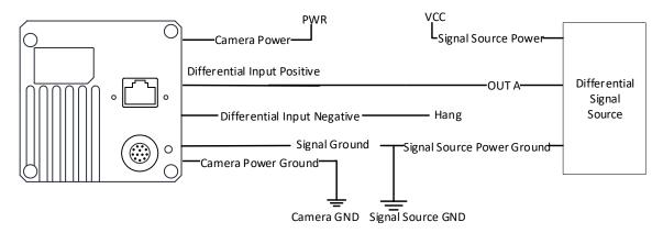
Figure 9-8 Differential Signal Source Outputs Single-Ended Signal
