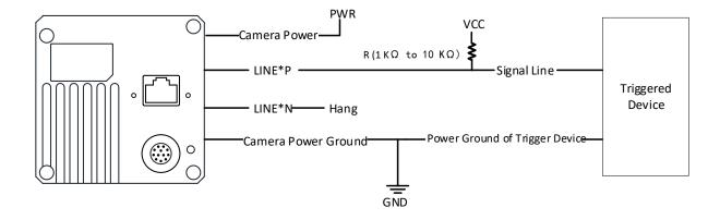
Figure 9-19 Single-Ended Output Wiring with Pull-Up Resistor
