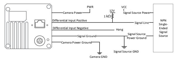
Figure 9-11 NPN Single-Ended Signal Source Connects Differential Input
