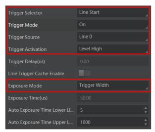
Figure 7-22 Trigger Width as Exposure Mode
