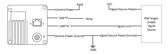
Figure 9-14 PNP Single-Ended Input Wiring without Pull-Down Resistor
