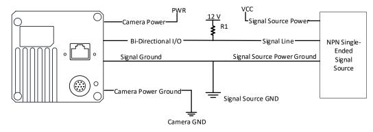
Figure 9-12 NPN Single-Ended Signal Source Connects Bi-Directional I/O
