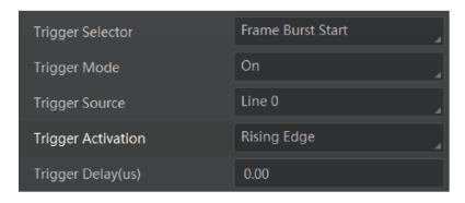
Figure 7-20 Edge Trigger in Frame Trigger
