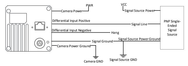
Figure 9-9 PNP Single-Ended Signal Source Connects Differential Input
