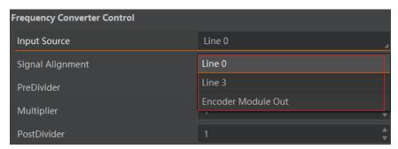
Figure 7-14 Set Frequency Converter Control
