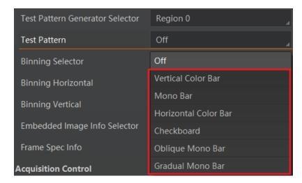
Figure 10-12 Test Pattern of Color Camera
