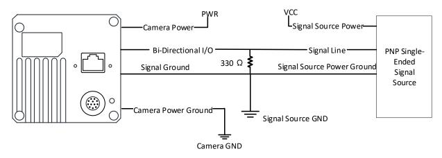
Figure 9-10 PNP Single-Ended Signal Source Connects Bi-Directional I/O
