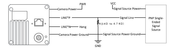
Figure 9-15 PNP Single-Ended Input Wiring with Pull-Down Resistor
