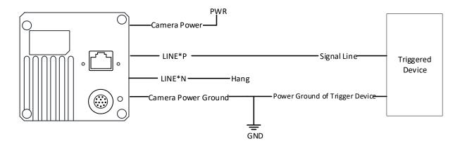
Figure 9-18 Single-Ended Output Wiring without Pull-Up Resistor
