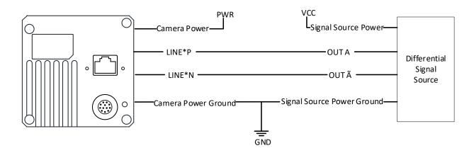
Figure 9-13 Differential Input Wiring
