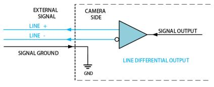
Figure 9-2 Internal Circuit of Differential output
