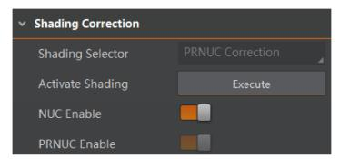
Figure 10-44 Set Shading Correction (I)
