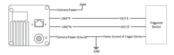
Figure 9-17 Differential Output Wiring
