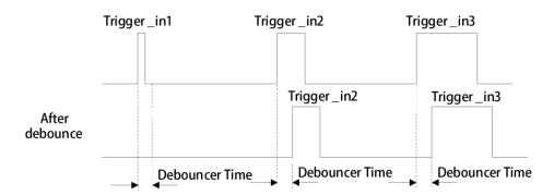
Figure 7-30 Trigger Debouncer Sequence Diagram
