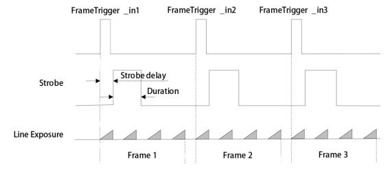
Figure 8-7 Sequence Diagram of Strobe Line Delay
