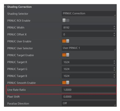
Figure 10-48 Set Line Rate Ratio
