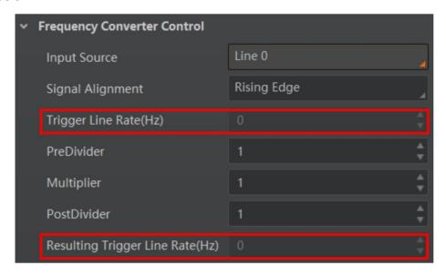
Figure 7-15 View Trigger Line Rate
