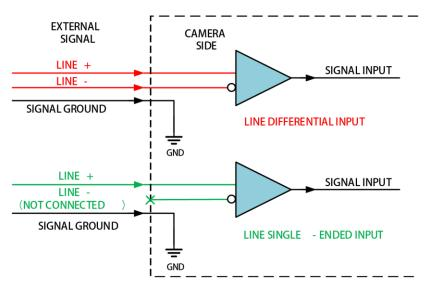
Figure 9-1 Internal Circuit of Differential Input
