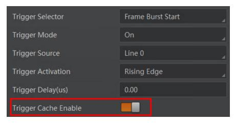
Figure 7-25 Set Trigger Cache in Frame Trigger
