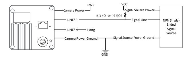
Figure 9-16 NPN Single-Ended Input Wiring
