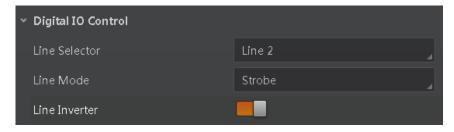
Figure 9-2 Enable Line Inverter
