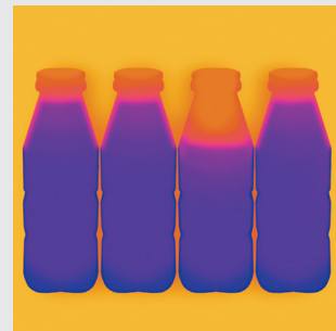
Detecting liquid levels in visually opaque bottles.
