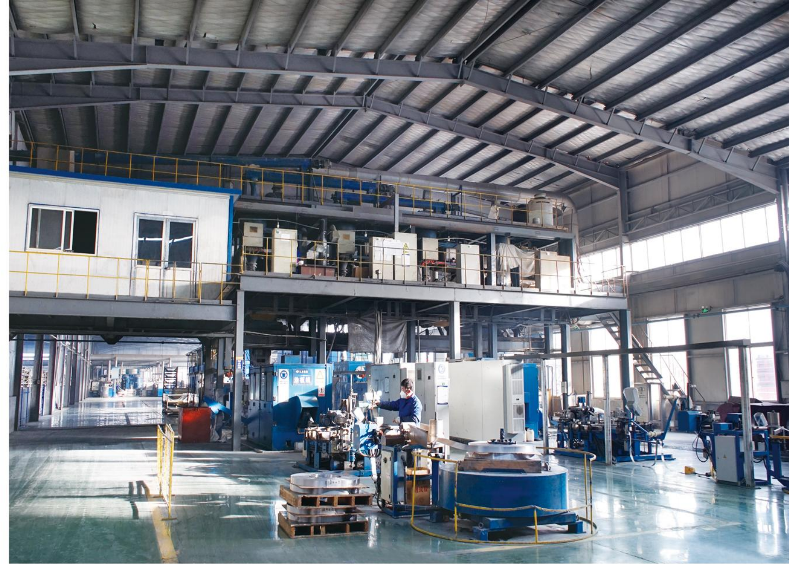
极板车间 Lead plate workshop (意大利索维玛扩网线 Italy Sovema cast & punch machine)
