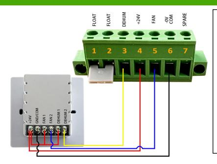
Connectiing the DHD100 digital control to the plug using a 4-core cable as the circuit diagram shows.
