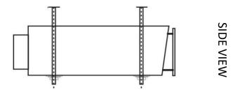
B. Install dehumidifier through the four thread rods, and adjust the height according the space to ensure the machine on horizontal level.
