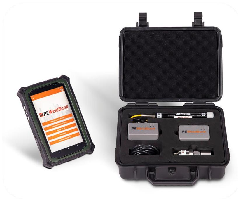
Data logger PEWeldBank is a fully-featured productivity and risk management tool that records weld data, calculates parameters for a wide variety of international standards, guides welders tutorial, weld assessment.
