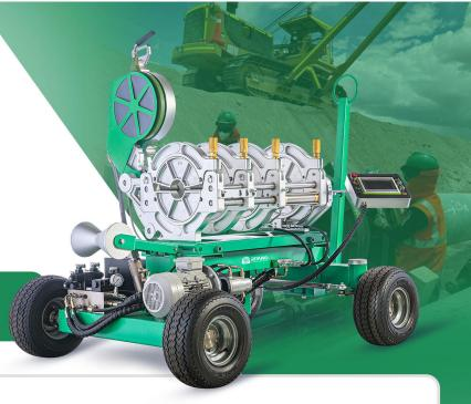
Riyang ARMOR 630i/24i is a high-performance fusion welding machine with trailer mobility, designed to excel on construction sites. It boasts a welding range from 315mm to 630mm or 12" to 24", adhering to ISO21307 and ASTM F2620 high-force standard. With a fully automated system featuring SIEMENS PLC technology, ARMOR 630i/24i ensures precision and reliability. Crafted from premium aluminum components, this machine guarantees strength and accuracy for all your welding needs.
