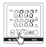
⑤ After setting, please press "SET" and then "INFO" to confirm. The value is memorized and the temperature controller rectifying automatically.
