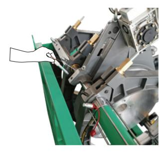
Rest the trimmer on the lower piston rod.
