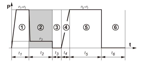
(Soaking pressure is needed to keep the two pipe ends in contact with the heating plate during this period.)
