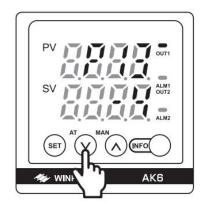
④ Press "SET" and "SV" will blink. Then set the value "-4" (if the actual temperature on heater surface is 4℃ higher than temperature set, set the value to be "4")
