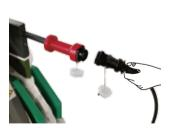
3. Connect heating plate cable to heating plate. It is connected properly only when sound "Click" made.
