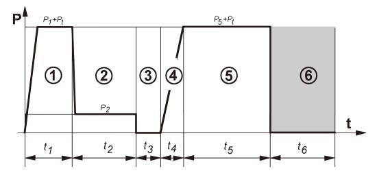
After time **T**<sub>5</sub>, release the pressure by rotating pressure relief valve in a counterclockwise way and remove the jointed pipe from the machine after time **T**<sub>6</sub>.
