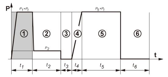
When the heating plate reaches the set temperature, insert it in between the two pipe ends. Close the pressure relief valve by rotating it in a clockwise way. And push the direction lever to close the carriage and keep the bead up pressure (P1+Pt) until the bead height reaches the requested one. Then release the direction lever slowly.
