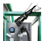
4. Connect heating plate cable to distribution box. It is connected properly only when sound "Click" made.
