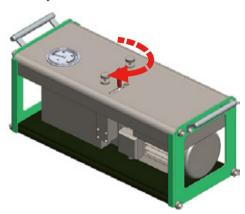
Then push the direction lever to maximum and gradually rotate the pressure regulated valve in a clockwise way, until the movable carriage gets in motion. Read the current pressure on the gauge and writ it down.
