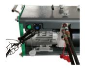
1. Connect power station cable to hydraulic station. It is connected properly only when sound "Click" made.
