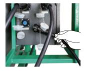
5. Connect the trimmer cable to distribution box. It is connected properly only when sound "Click" made.
