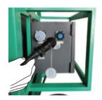
2. Connect power station cable to distribution box. It is connected properly only when sound "Click" made.
