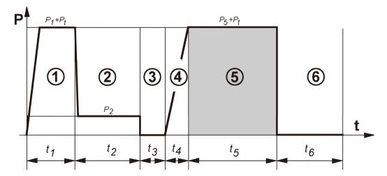
To stabilize the pressure  $(P_5+P_t)$ , please keep the direction lever pushed for around 10seconds. Then release the direction lever slowly. Wait  $T_5$  time to end.
