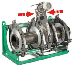
When the continuous and even chip comes out from both pipe ends, stop the motor by pressing the stop button(red button).
