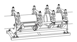
The dragging pressure must be measured with pipes/fittings clamped.
