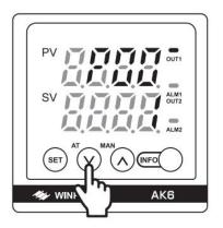
③ Press "SET" and "PV" will blink. Press "V" or "A" until the "PV" value shows "P13"
