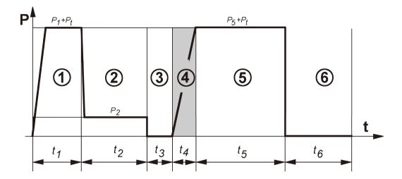
Close the pressure relief valve, and push the direction lever to maximum , meanwhile gradually increasing the pressure until the pressure gauge reaches the welding pressure  $(P_5+P_t)$  , within  $T_4$  time.
