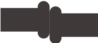
Misalignment. Welding under the condition that the misalignment exceeds 10% of pipe wall thickness while align the two ends.
