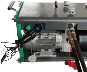
Connect power station cable to hydraulic station. It is connected properly only when sound "Click" made.
