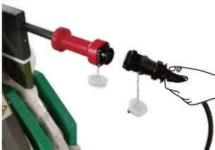
Connect heating plate cable to heating plate. It is connected properly only when sound "Click" made.
