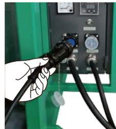
Connect power station cable to distribution box. It is connected properly only when sound "Click" made.
