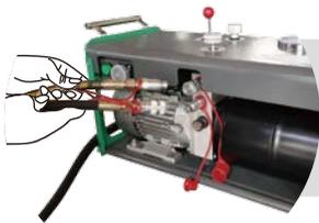
Connect the hydraulic hoses to hydraulic power unit.
