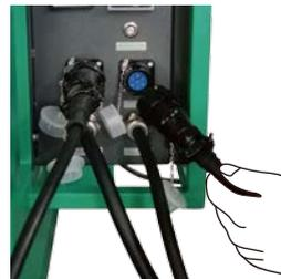
Connect the trimmer cable to distribution box. It is connected properly only when sound "Click" made.
