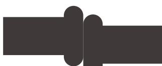
Misalignment. Welding under the condition that the misalignment exceeds 10% of pipe wall thickness while align the two ends.
