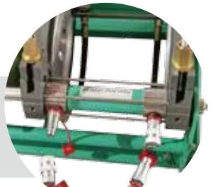
Connect the hydraulic hoses to machine carriage.
