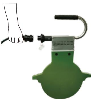
Connect heating plate cable to heating plate. It is connected properly only when sound “Click” made.
