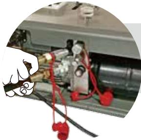
Connect the hydraulic hoses to hydraulic power unit.
