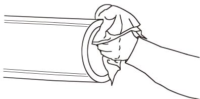
Be sure the internal and external surfaces of the pipe ends be cleaned well.
