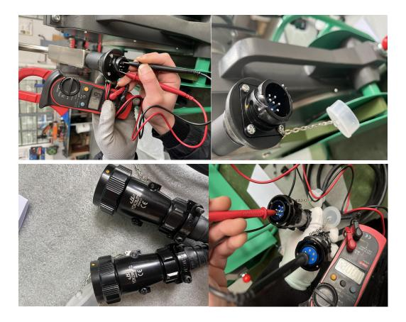
Before troubleshooting, ensure that the power supply voltage and all connections are correct, and that there is no surface damage. Repairs must be performed by professionals only!
