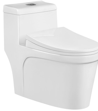
Model: A3931 One piece toilet (Siphonic) Size: 725x400x650mm S-trap: 300/400mm
