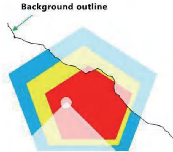
**Main point** When the monitoring zone group selection mode is set to "I/O input", the "background trimming" function of the activated monitoring zone group is automatically enabled.
