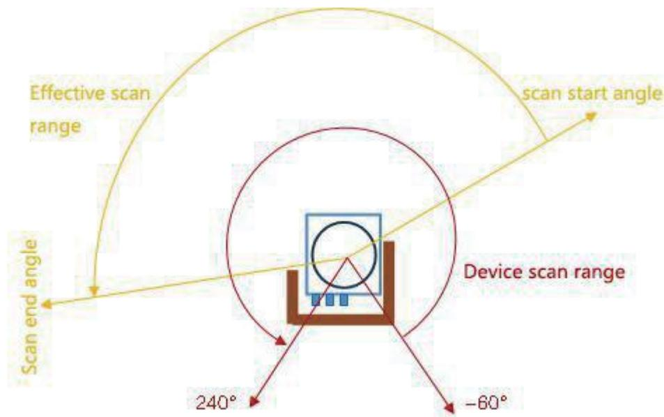
You can use FILPS software to adjust the TOF-20Ss scan start angle and scan end angle as follows:
