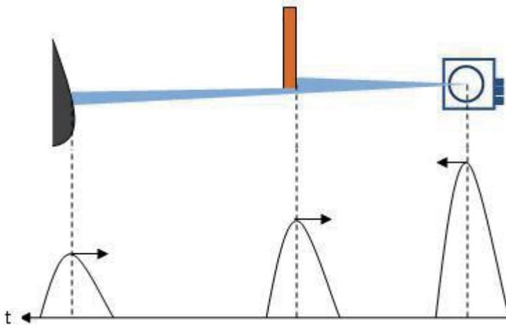
If the distance between the target and the background is close, the two echo echoes will overlap each other, which will lead to the inaccuracy of the measurement and the "pseudo edge point", which is far farther away than the actual distance from the target edge, as shown by the "Figure 4.2 pseudo edge point". The difference between the measured values and the real values of the pseudo edge points may reach 15cm.
