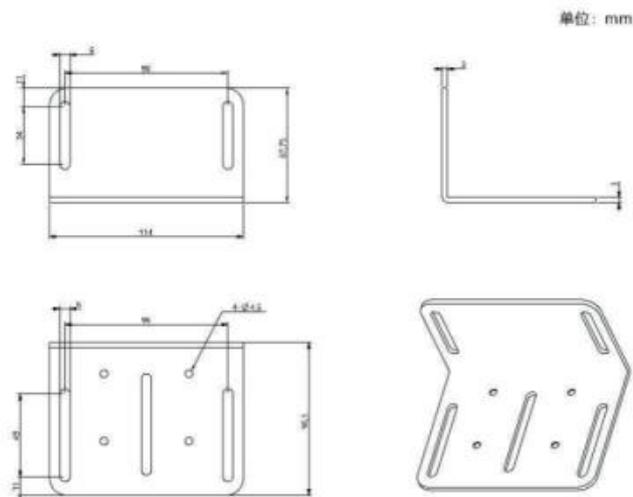
Figure 10.4 Assembly Drawing of TOF-20S-AT
