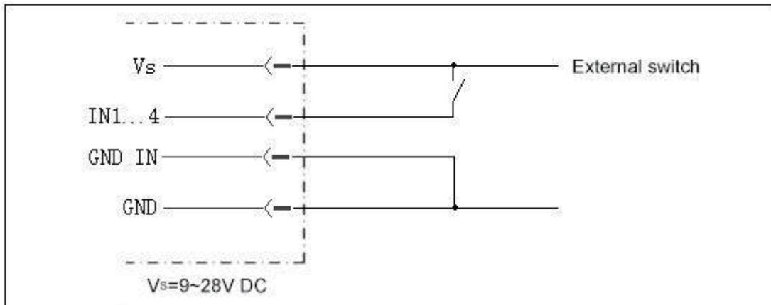
Figure 6.2 I/O Interface Input Terminal External Circuit (Floating)
