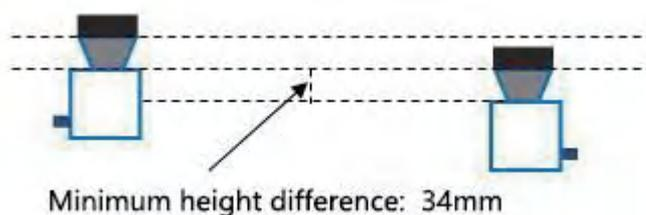
Figure 5.3 Adjustment of pitch angle of scanning surface
