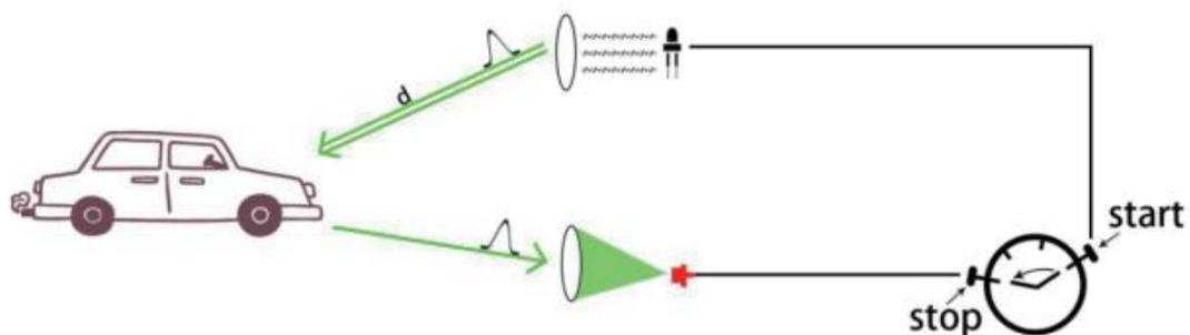
TOF-20S has multiple echo analysis capabilities. In the rain and fog and soot working environment, atmospheric impurities will also reflect the distance measuring laser pulse, forming a reflected echo pulse, and together with the reflected echo pulse of the measured target, reach the photoelectric receiving system. The TOF-20S analyzes all received reflected echo pulses, rejects interfering pulses, and outputs true measured target distance data, as shown in Figure 3.3 Reflected Echo Filter.
